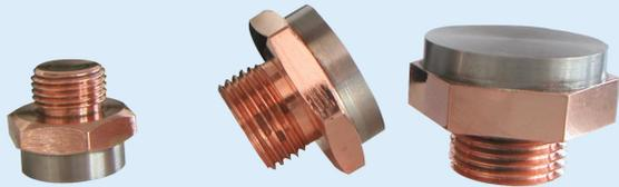
We manufacture Tungsten Copper faced projection Welding Electrodes for nut welding. The increased wear resistance of Tungsten Copper facing offers enhanced working life of electrode and less frequent replacements. Our electrodes are the benchmark for quality in the industry as we control all operations inhouse like sintering, brazing and CNC machining. This gives us the start to finish control we need to achieve High Quality.
