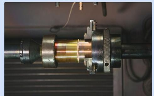
Electron Beam Welding
